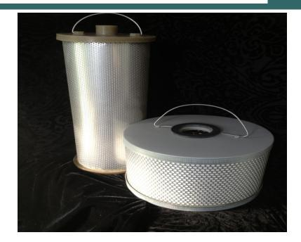
Jaxon's *Trans-Dri* filter element is designed to remove free and dissolved water from insulating oils. Moisture can be lowered to less than 10 PPM without the use of heat and vacuum processing.
